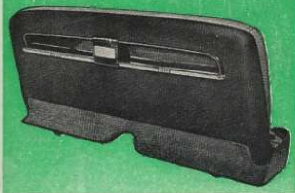
A handy feature on the '49 Nash is this magazine or map rack on back of front seat. It's about 2½" deep
