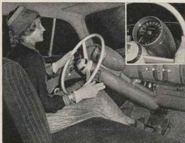
Left, mounted on massive steering column is cockpit-type instrument group. Below, pickup pump on carburetor acts to smooth fuel flow with engine demand
