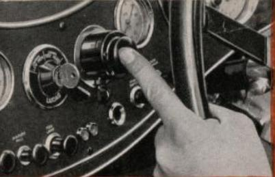
All controls fall readily to hand; dipper switch, horn, etc., can be operated without removing a hand from the steering wheel.
