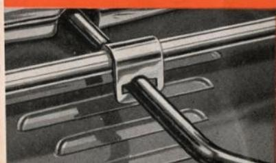
A badge bar is part of the standard equipment; it carries a fog lamp and horn and a centre bracket locates the starting handle.
