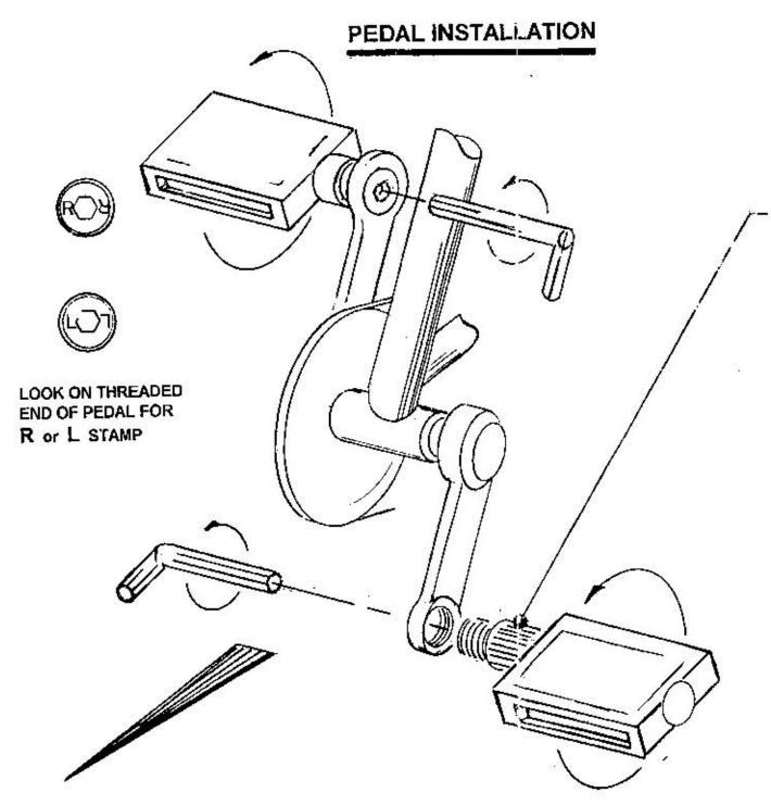
INSTALL RIBBED SHAFT PEDAL TO LEFT SIDE OF BICYCLE
