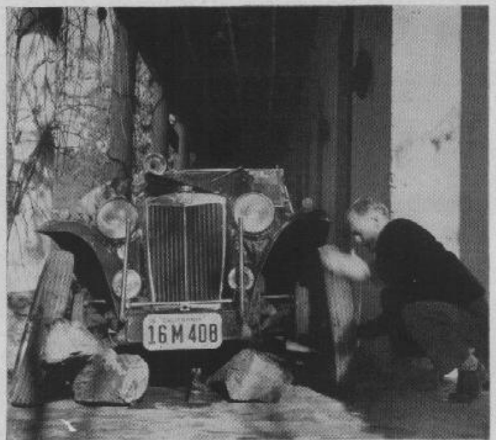
WHEEL-CHANGING technique is shown by Club Organizer Bjarne Qvale. Hubcaps which can be "knocked off and on" permit three-minute wheel change.
